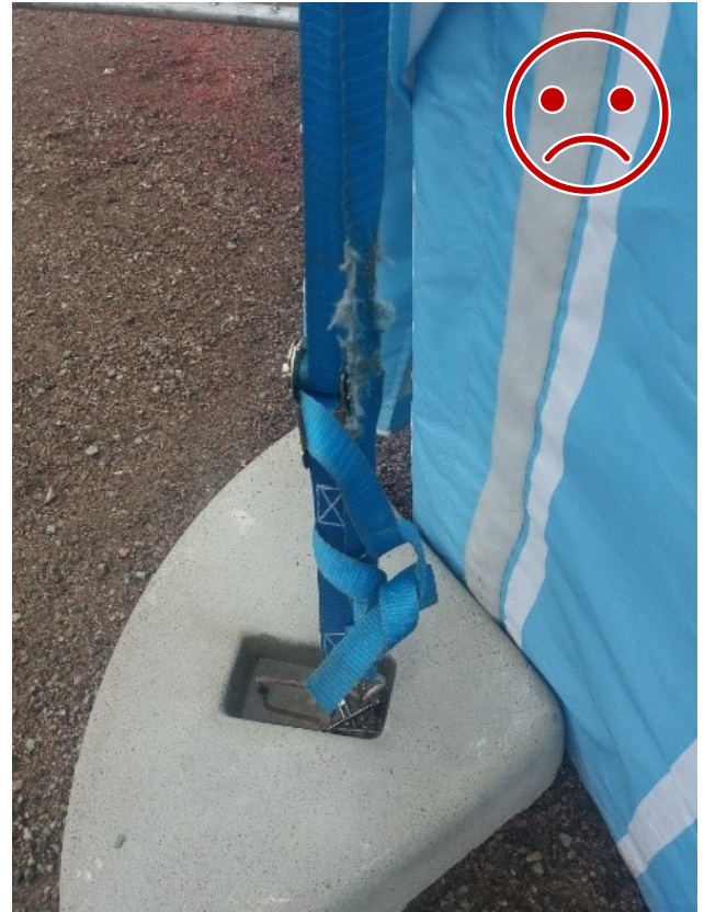
Figure 10 WRONG . The strap is worn.
